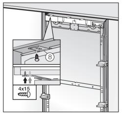
Screw the attachment plate lugs (8) to the overhead furniture/fixtures.
